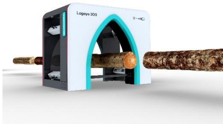
Logeye Fingerprint 3D + Xray scanning
