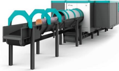
CT Log Full 3D internal defect scanning
